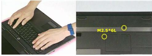
OPTICAL DRIVE MODULE INSTALLATION
