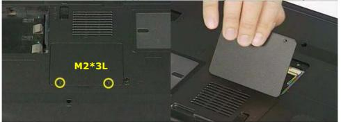
2. Insert the new memory module to DIMM socket at 45 degrees angle and push it down to lock it up. Put on the memory DIMM cover and secure 2 screws (M2\*3L(K)) to fix it.
