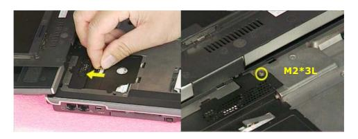
8. Install the keyboard cover then secure 2 screws (M2\*3L(K)) to fix it.
