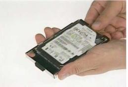
5. Secure 2 screws (M2\*4L) on both sides
