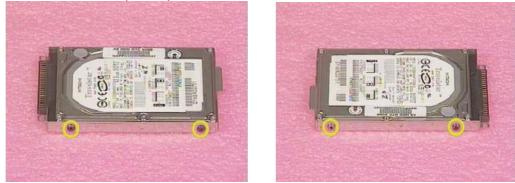
6. Insert the hard disk moudule into its compartment and lay it down gently then put on the hard disk cover. And secure 2 screws (M2\*6L(K)).
