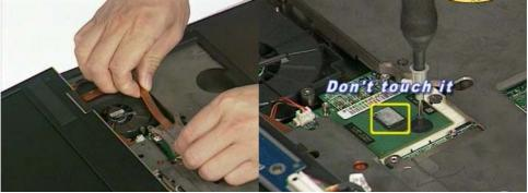
6. Insert the new CPU onto the socket then close the CPU Socket's latch to fix it.
