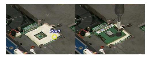
7. Paste thermal pad onto the CPU heat sink module then install it.
