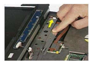
10. Install the keyboard cover then secure 2 screws (M2\*3L(K)) to fix it.
