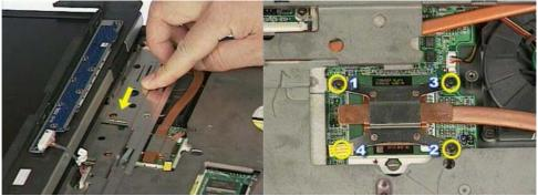
5. Remove Thermal module and open the CPU Socket's latch to loosen the CPU.(The use the CPU vacuum hand pump to "suck up" the CPU and lift the CPU away.)
