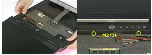
9. Install the keyboard module onto top case and secure 2 screws (M2.5\*6L(K)) at bottom side then fix it.
