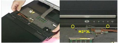
11. Install the keyboard module onto top case and secure 2 screws (M2.5\*6L(K)) at bottom side then fix it.
