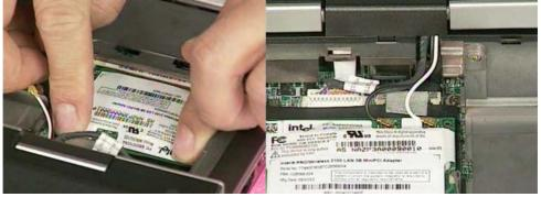
7. Put on the mini-PCI cover and secure 1 screw (M2\*3L(K)) to fix it.
