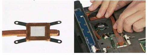
8. Secure 4 screws to fix it and stick the warranty seal label on the screw.
