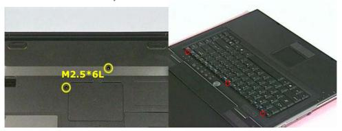
2. Pull out the keyboard module and then lay on the top case. Disconnect keyboard FPC cable and take the keyboard away.
