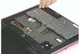
3. Remove 2 screws (M2\*3L(K)) at keyboard cover and use tweezers to lift up the keyboard cover's two nooks.
