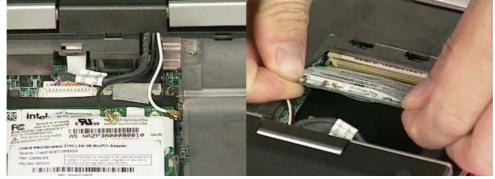
6. Insert the new wireless LAN module to mini-PCI socket at 45 degrees angle and push it down to lock it up and connect the 2 antenna cables.
