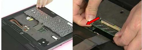
3. Insert the new memory module to DIMM 45 degrees angle and push it down to lock it up. Install the keyboard module onto top case and secure 2 screws (M2.5\*6L(K)) at bottom side then fix it.
