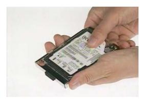
4. Replace the new Hard-Disk onto the HDD Housing.
