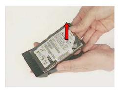
3. Place new HDD into the HDD housing. Secure 2 screws (M3\*3L) . Then 2 screws (M3\*3L) on the other side.
