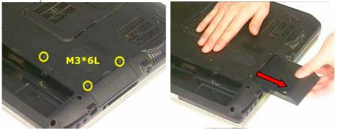
2. Remove 2 screws (M3\*3L). Then on the other side 2 screws (M3\*3L). Then separate HDD from the HDD Housing.
