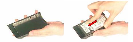
**4.** Replace HDD Module, and Secure 3 screws (M3\*6L) . This completes the HDD installation and replacement.
