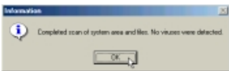
(3) Wait while your setup checks your system for viruses based on the included pattern file. (This is usually older than what is available on the Internet at "http://www.trend.com". You should rescan your hard drives after updating the virus pattern.) Click OK when completed.
