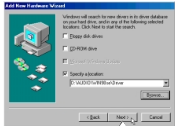
(11) Enter the letter of your CD-ROM drive and the AUDIO\WIN9X\DRIVER path on the Notebook PC support CD. (Browse to the folder that corresponds to your OS.) Click Next to determine the best driver for your device.
