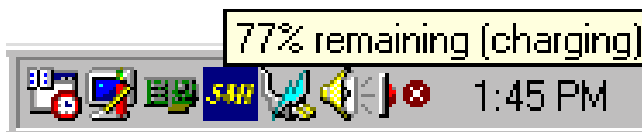
Power icon using AC power. The charging (lightning) icon appears if the battery is not fully charged.
