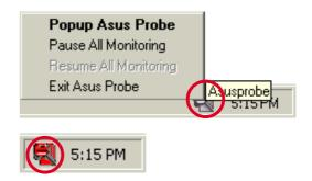
**NOTE:** PC Probe will constantly use resources to check the system status while Windows is operating. It is suggested to exit PC Probe while using high demanding applications.
