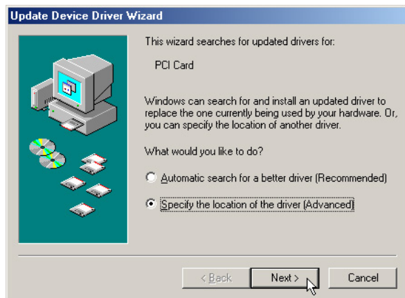
(4) This installs the first driver. Select "Specify the location..." and click Next .
