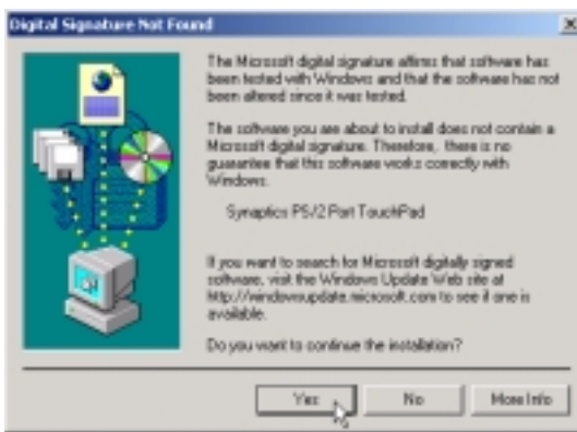
(4) Click Yes to accept the driver because the driver on this support CD has been fully tested by the Notebook manufacturer to work correctly with MS Windows.
