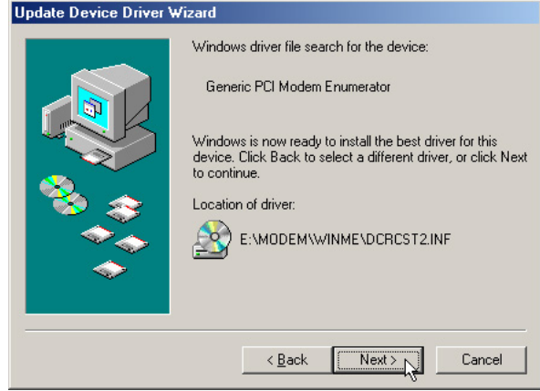
(6) Verify that the location of the driver is from the support CD. Click Next to install.
