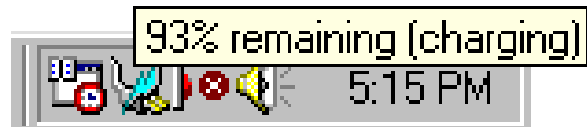
Power icon using AC power. The charging (lightning) icon appears over the “plug” icon if the battery is not fully charged. When fully charged, only the “plug” icon will remain.
