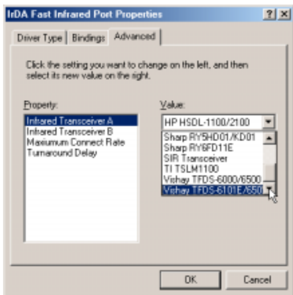
(13) Click Advanced tab and select Vishay TFDS-6101E/6501R for “Infrared Transceiver A” and click OK .
