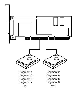
In RAID 1, MegaRAID SCSI 320-0 duplicates all data from one drive to a second drive. RAID 1 provides complete data redundancy, but at the cost of doubling the required data storage capacity.
