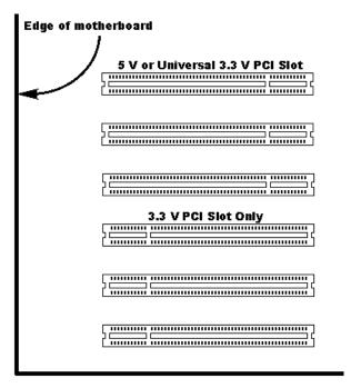
Insert the MegaRAID SCSI 320-0 card in the ZCR PCI slot as shown below. Screw the bracket to the computer frame.
