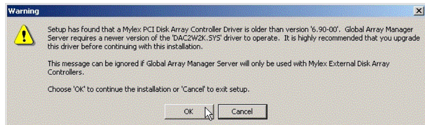
Figure 3.7 Error – PCI Driver Must Be Version 6.90-00 or Higher
