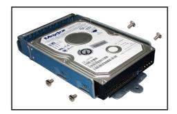
Carefully place the tray with installed hard disk drive into the drive bay. Slide it forward until the front end aligns with the front panel, and the screw hole matches the standoff.
