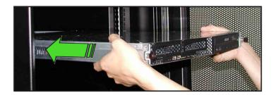
2. Carefully push the server all the way to the back until the front panel fits the front end of the rack, and the rack screws on the server match the middle hole on the rack.
