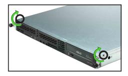
2. Loosen the two thumbscrews on the rear panel to release the top cover from the chassis.
