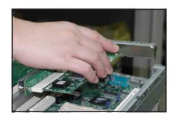
When properly installed, the riser card brackets with PCI cards appear as shown.
