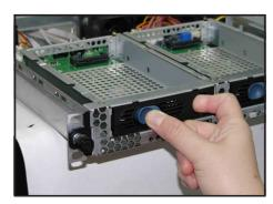
2. Firmly hold the tray lever and pull the drive tray out of the bay.
