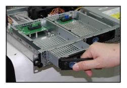
3. Take note of the drive tray holes. Each side has three holes to fit different types of hard disk drives. Use two screws on each side to secure the hard disk drive.
