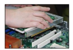
If you wish to install a second PCI card, repeat steps 1 and 2 then install the card to the right bracket as shown. Secure the card with a screw.
