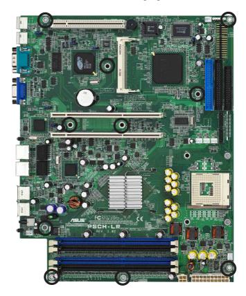
4. Carefully lift the motherboard out of the chassis.
