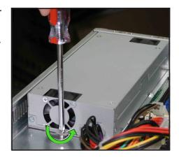
3. From the rear panel, remove the two screws the secure the rear end of the power supply.
