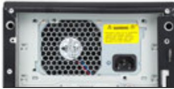
600 W single power supply (110 V / 220 V autoswitch)
