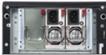
2 x 300 W dual power supply (110 V / 220 V autoswitch)
