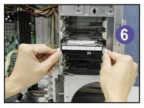
6. Connect one end of a 40-pin IDE cable to the IDE connector on the drive. Connect the other end to an availble IDE connector on the motherboard.
