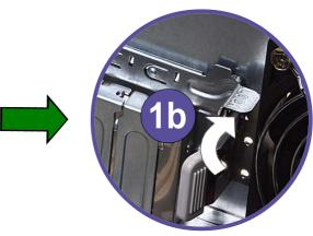
Slide out the metal bracket opposite the PCI slot where you wish to install the expansion card. You may use a flat-head screwdriver to easily remove the bracket.
