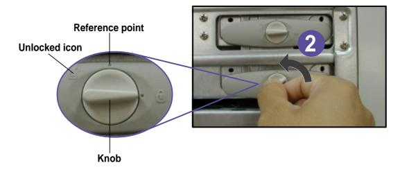
3. When released, pull out the drive bay lock and set it aside.
