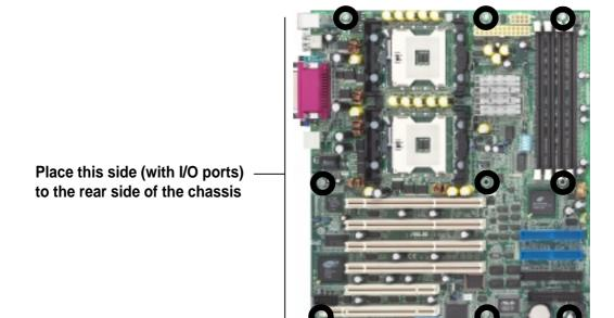
The following figure shows the specific locations of the standoffs (indicated by black circles) inside the chassis. These standoffs should match with the holes on the motherboard as pointed out above.
