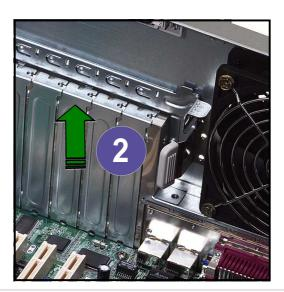
3. Install the expansion card making sure that it is properly seated on the slot.
