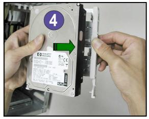
5. Carefully insert the drive tray into the bay until you hear a click indicating that the tray is in place. The drive tray is correctly placed when its front edge aligns with the bay edge.
