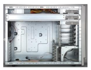
The chassis supports an extended ATX form factor ASUS motherboards. See the motherboard dimension requirements on page 2-4.
