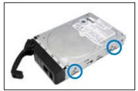
Carefully insert the drive tray and push it all the way to the depth of the bay until just a small fraction of the tray edge protrudes.
