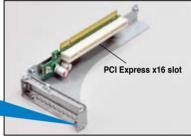
Install a PCI Express x16 card to the bracket as shown, and then secure the card with a screw.
