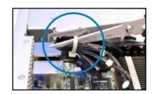
Connect the SGPIO cable to the SGPIO1 connector into the SGPIO2 connector on the PIKE riser card.
