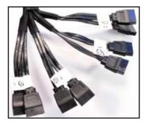
Connect the SATA/SAS cables to the SAS1–8 connectors on the PIKE riser card.
