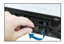
Take note of the drive tray holes. Each side has three holes to fit different types of hard disk drives. Use two screws on each side to secure the hard disk drive.
