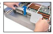
Connect the red end of the 8-pin power cable to the power connector on the GPU computing module.
