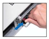
3. Firmly pull the PSU out of the system chassis.
