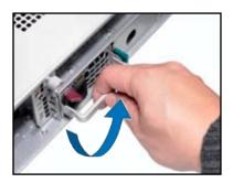
2. Hold the PSU lever and press the PSU latch.
