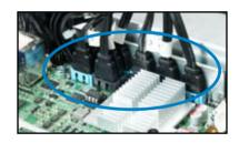
The SATA/SAS cables are tied and labeled in four groups. Group 1 connects to HDD 1 and 2, Group 2 to HDD 3 and 4, Group 3 to HDD 5 and 6, and Group 4 to HDD 7 and 8.
