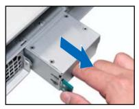
3. Insert the PSU into the empty PSU bay.
