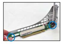
3. Locate the two screw holes on the PIKE riser card.
