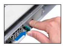
2. Firmly pull the PSU dummy cover out of the server chassis.
