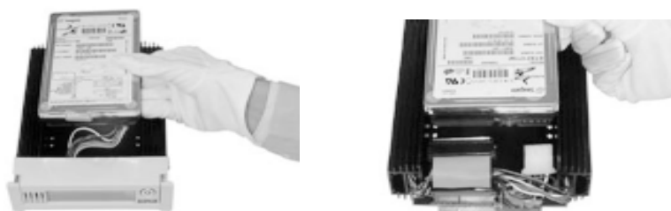
Fig 3-24: Necessary Cables Connect to SCSI device both Front and Back.
