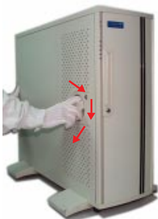
Fig 3-17: Lock the cover
