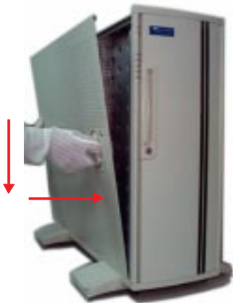
Fig 3-16: Replace the cover
