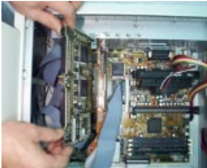
Fig 3-12: Insert a VGA/ PCI add-on card
