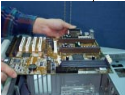
Fig 3-6: Place the motherboard
