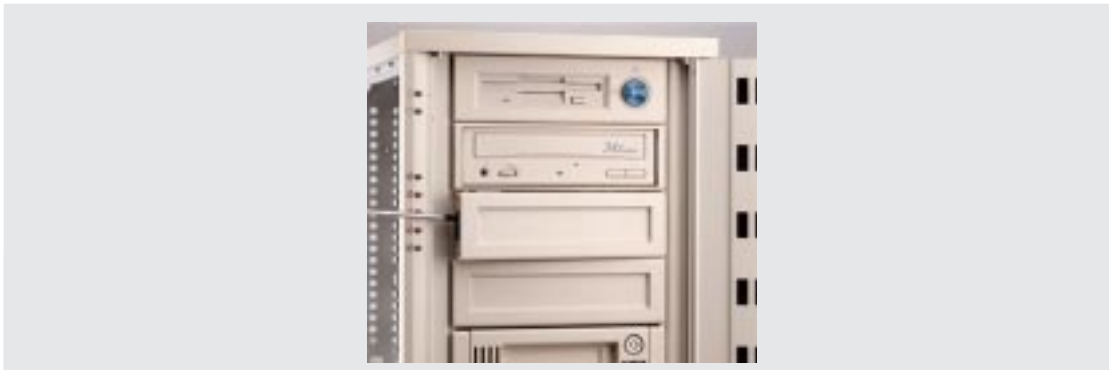
Removing the device bay cover
