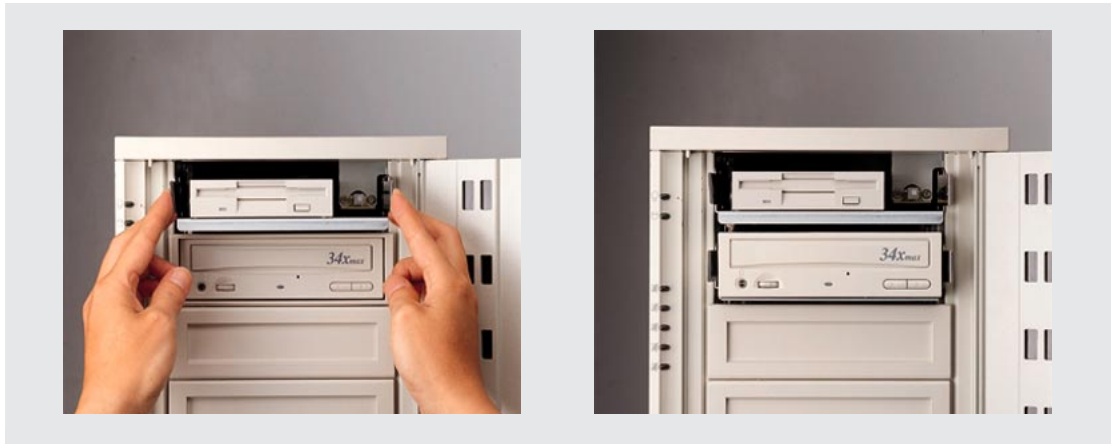
Removing Floppy and CD-ROM device
