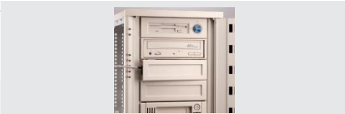
Removing the device bay cover
