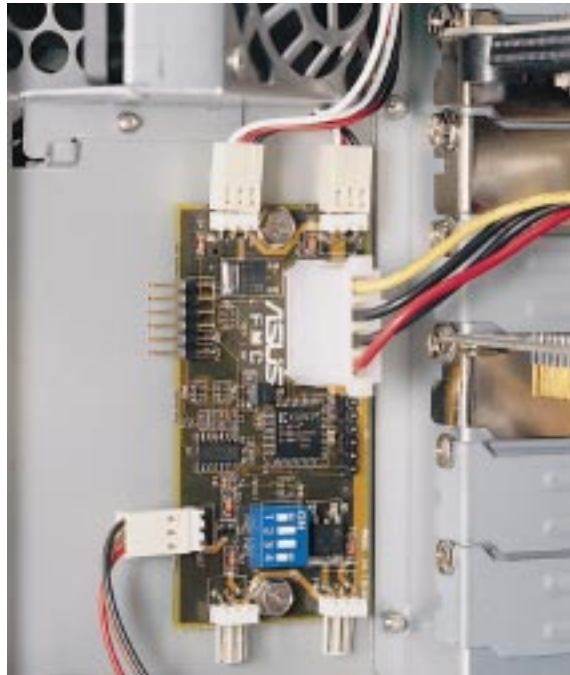
Fan control board with cable connections
