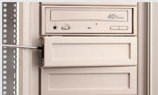
Removing the device bay cover clips
