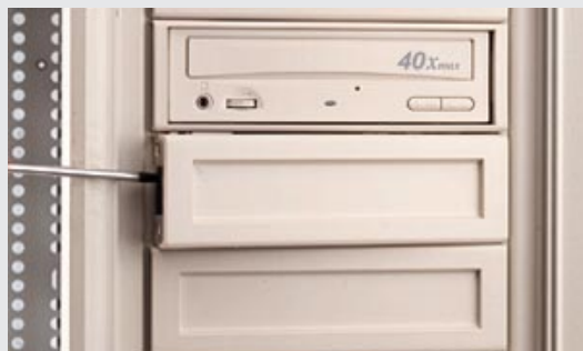
Removing the device bay cover clips
