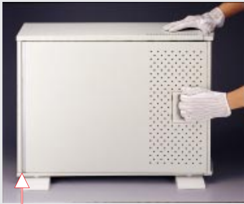
Pulling the panel forward
