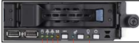
HDD Access LED LAN2 LED LAN1 LED Message LED Location LED Power LED
