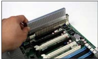
3. Insert the RAID card into the PIKE RAID card slot. Ensure that it is completely seated on the PIKE RAID card slot.
