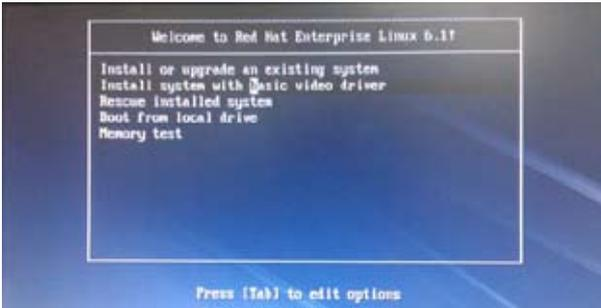
3. At the boot:, type `vnlinux initrd=initrd.img xdriver=vesa nomodeset dd` , then press <Enter>.
