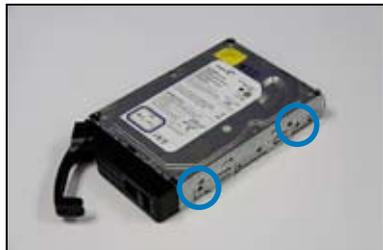
5. Carefully insert the drive tray and push it all the way to the depth of the bay until just a small fraction of the tray edge protrudes.
