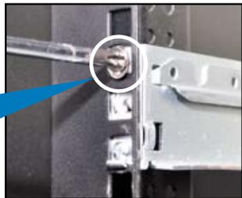
6. When mounting the server to the rack, ensure to include the side knots on the two sides of the server in the rack rail holders, as shown in the right figure.
