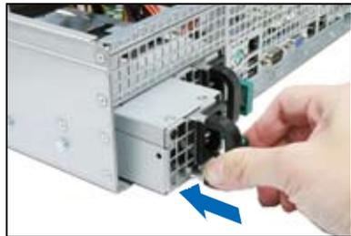
3. Firmly pull the lever to slide the power supply module into the chassis.
