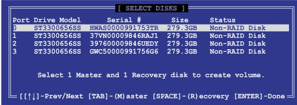
5. Use the up/down arrow keys to select a drive, press <TAB> to select a Master disk, and then press <SPACE> to select a Recovery disk. A small triangle marks the selected drive. Press <Enter> after completing your selection.
