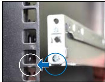
4. Secure the front and rear ends of the rail with two rack screws and washers.
