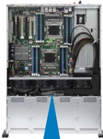
Connects to the SAS connectors on the motherboard. Install an optional ASUS PIKE SAS RAID card or a 3rd party RAID card before using these ports.
