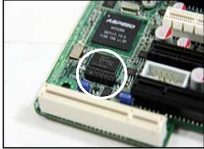
2. Place the board on the ASMB6 connector of the motherboard, aligning with the pin connectors.
