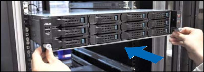
2. Tighten the two rack screws to secure the server in place.
