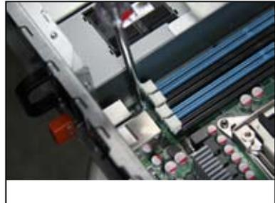
3. Place the airduct on the motherboard, ensuring that the three fasteners match the holes on the motherboard.
