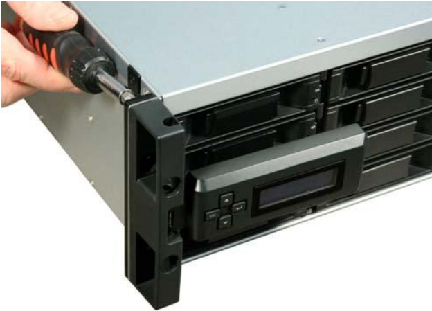
Figure 5. Attach the LCD panel to the ASUS Storage enclosure
