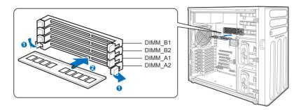
You may install 1GB, 2GB, 4GB and 8GB Unbuffered with ECC DDR3 DIMMs into the DIMM sockets using the memory configurations in this section.
